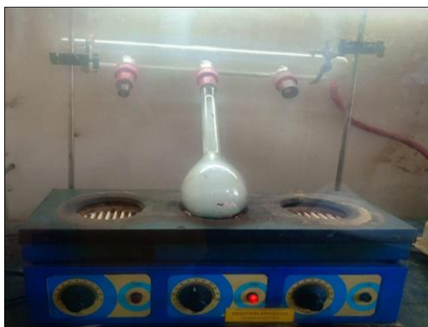
Fig 5: Protein analysis by Kjeldahl method
