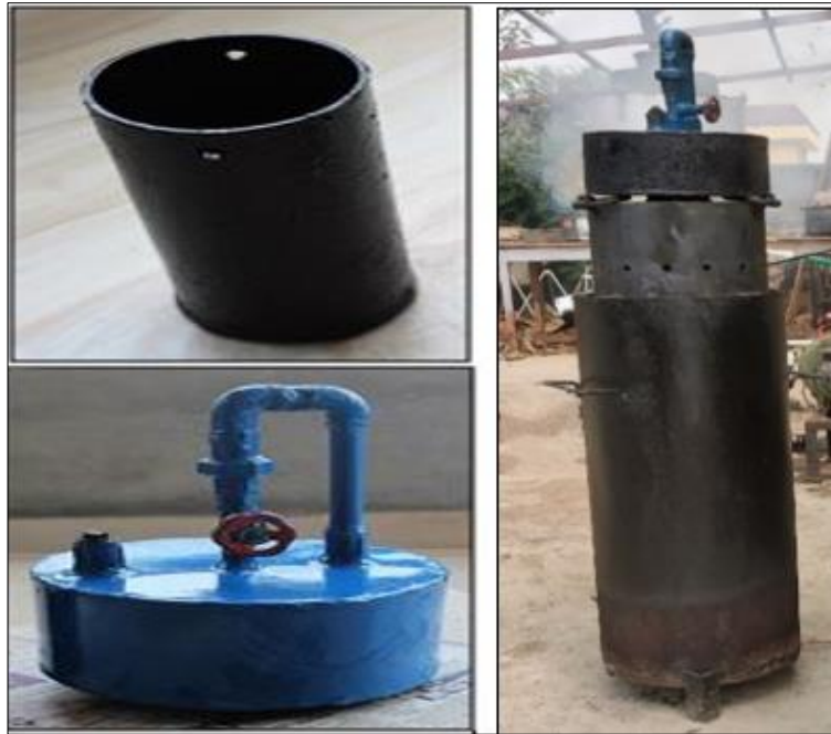
Fig 2: Pictorial view of existing open top gasifier and developed steam activation unit
