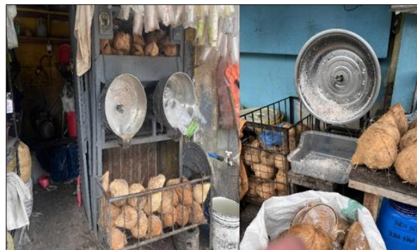
Fig 1: Coconut grater machine powered by 1Hp motor
