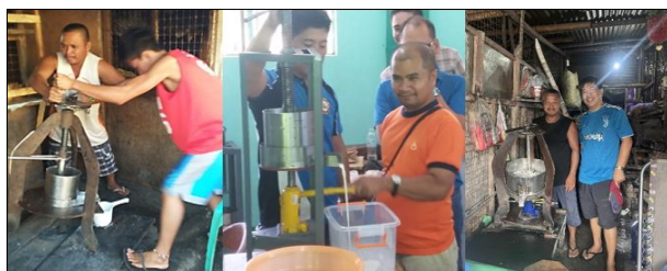
Fig 4: Innovation transformation from screw press to screw and hydraulic coconut milk extraction
