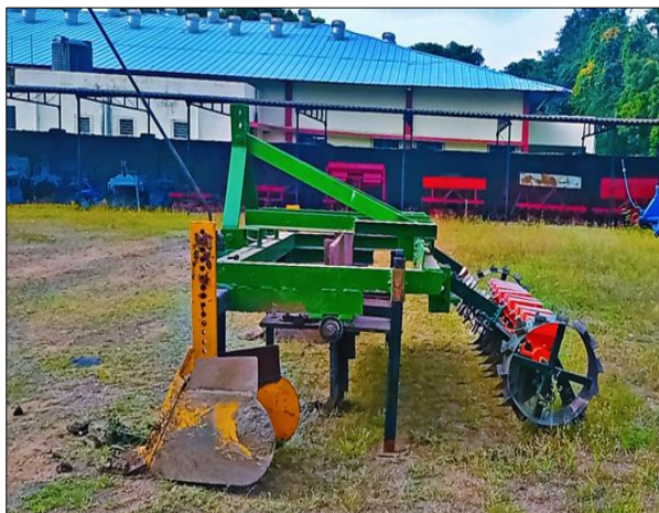
Fig 1: Light weight multi crop basin lister seeder
