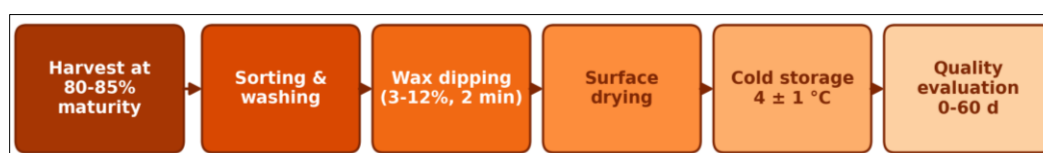
Fig 3: Process diagram of wax coating and cold storage workflow for Clemenules mandarin from harvest to quality evaluation
