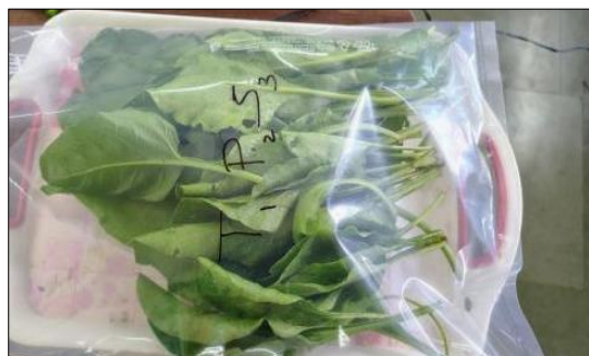
Fig 7: Packaging treatment of non-perforated LDPE packaging
