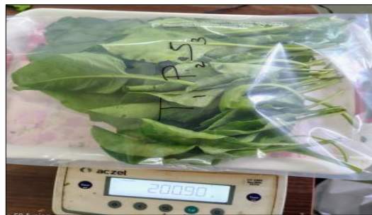
Fig 8: Packaging treatment of perforated LDPE packaging
