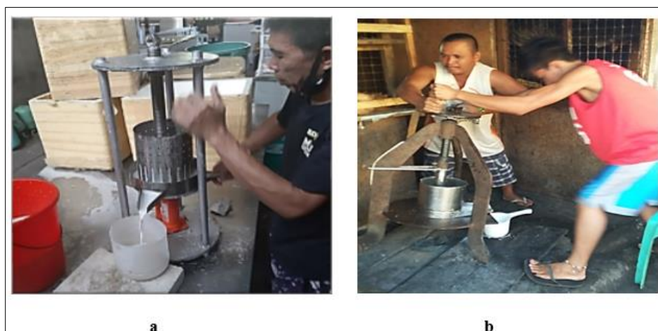
Fig 5: Coconut milk extraction using a. the coconut milk extractor, b. screw press
