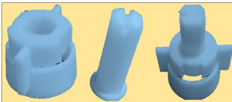
Fig 7: 3D Prototype model of nozzle extruded from 3D Stratasys Printer
