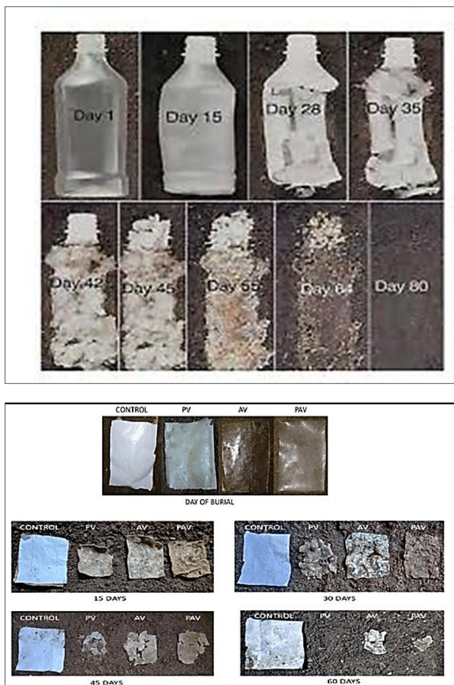
Fig 8: A. Biodegradable PHA bottles (Diederik van der Hoeven, 2016). B. Biodegradable films (Krishnamurthy et al. 2019 [13, 24])
