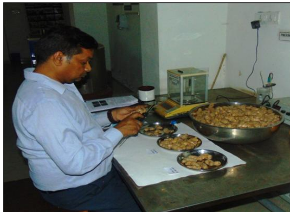
Plate 5: Measurement of axial dimensions of turmeric rhizomes for grading
